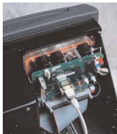
The manifold assembly, with supporting circuitry, mounts against the front panel of the FastPack.
