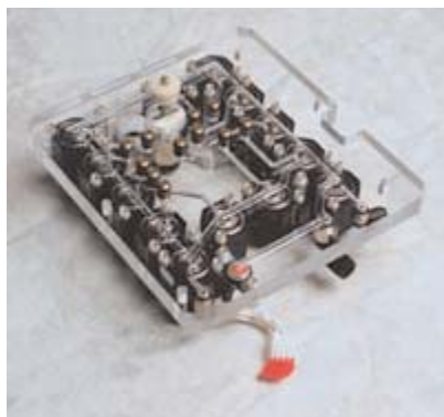
Thirteen Clippard ES-3T-12 valves mounted on an acrylic manifold feed compressed air to actuators (brass color, with O-rings) that move liquids within the sample pouch.
